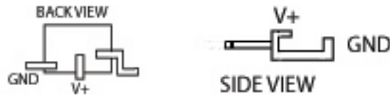
Figure E-4: Power connector to the housing of the connector on the iPAQ side and power connection for the charger.
