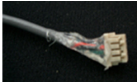
Figure E-5: A completed wireless receiver cable to connect to the wireless receiver.
