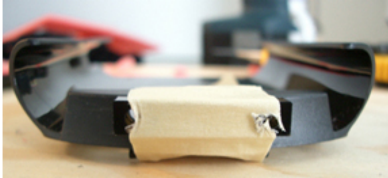
Figure E-7: The drill template attached to the sleeve jacket to direct the placement of the holes.
