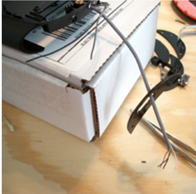
Figure E-10: Stringing the cable through the necessary parts in order to create the housing.
