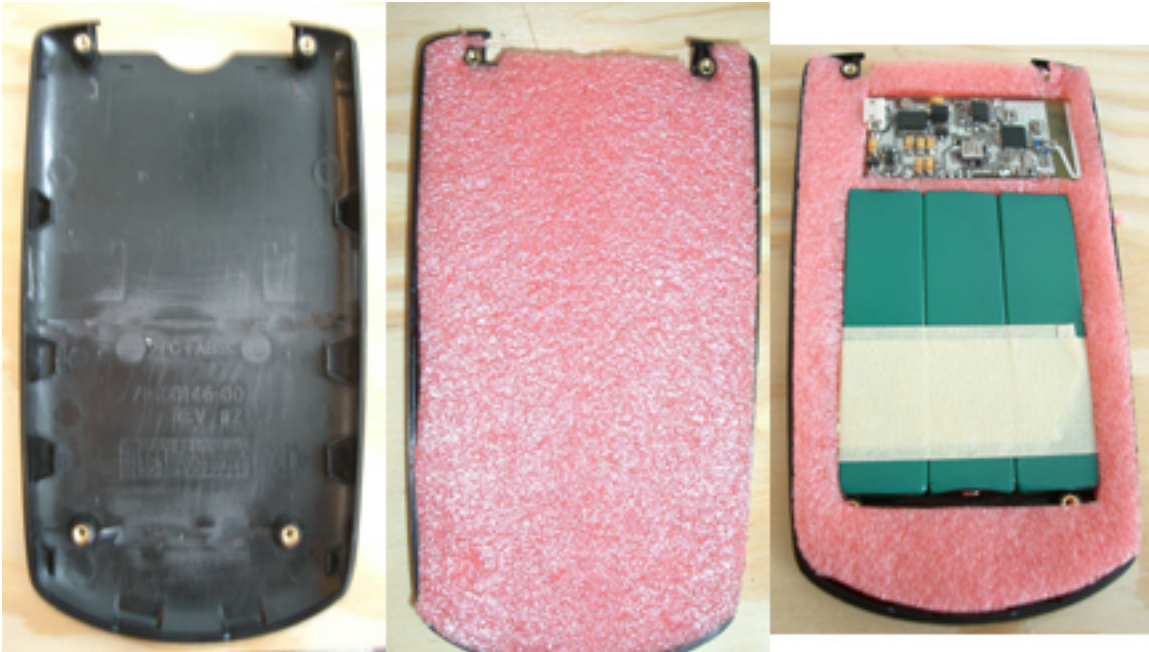
Figure E-6: Starting from the left: a sanded interior of the cover, foam cut to fit the inside cover, and the finished cover
