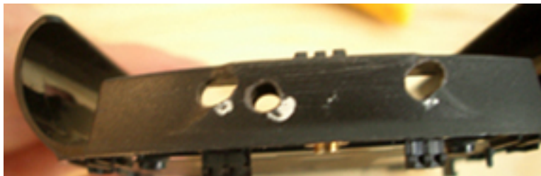
Figure E-8: The sleeve jacket with the 3 holes needed for the cable connector.
