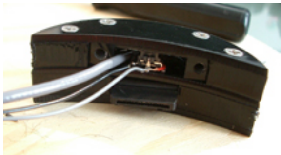
Figure E-12: A completed connector housing before it is attached to the jacket.
