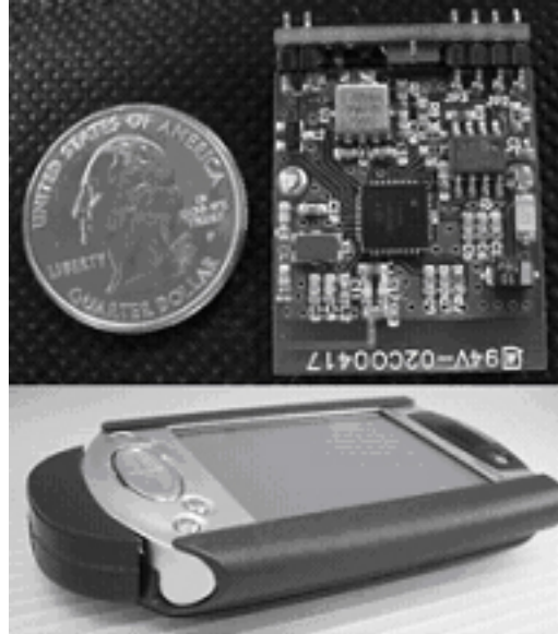
Figure 3-3: The 3-axis wireless accelerometer (top) and the iPAQ with the receiver casing (bottom).
