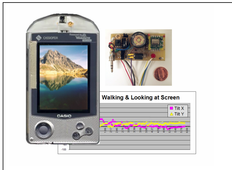
Figure 7. Sensing PDA, outfitted with multiple perceptual sensors, including proximity, motion, and touch sensors. In the background, accelerometer signals are displayed showing the motion fingerprint of a user walking while looking at the device.
