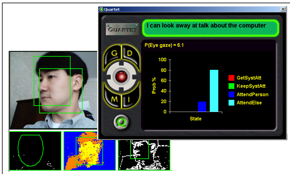
Figure 9. Quartet in action. Quartet's partial recognition is displayed at the top of the display. The system's beliefs about the attentional status of the user, with regards to initiating, maintaining, or breaking out of conversational dialog, is represented as a dynamically changing probability distribution.
