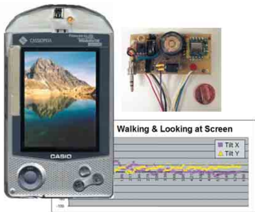
Figure 4. Sensing PDA, outfitted with multiple perceptual sensors, including proximity, motion, and touch sensors. In the background, accelerometer signals are displayed showing the motion fingerprint of a user walking while looking at the device.
