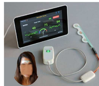
Fig. 1. Neurosteer EEG system. A wearable one-lead medical electrode with a single-use sensor that attaches to the forehead and a relay computer connected to the Neurosteer® Cloud server.
