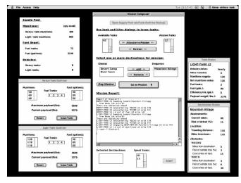
Figure 1: The Tank Task used in the experiment. The upper left window lists available resources. The two windows on the bottom left allow the user to outfit heavy (middle) and light (lower) tanks. The two windows on the right show the stats for a selected tank (middle) or city (lower). The large window in the center provides information about cities, missions, and mission outcomes.
