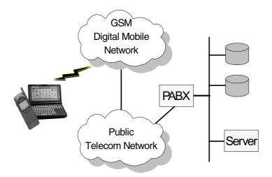
Key features of this architecture are that mobile clients can access data on the LAN, and that access to the system is possible using existing telephones via the PABX. The communication application features include:
