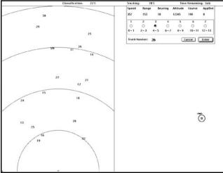
Screen shot of Argus Prime from Study 2. Radar display is on left-side. Operator position is represented by the small + at the bottom left. The flying numbers represent planes. Right-side shows information window at top with information on the currently selected target. Bottom right shows the randomly moving target and the cursor with which the operator is supposed to track the target.
