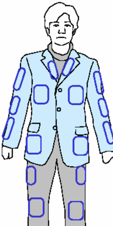
Figure 13. GesturePad—a wearable input method. The dark blue outlines show areas that are sensitive to touch (Rekimoto 2001).
