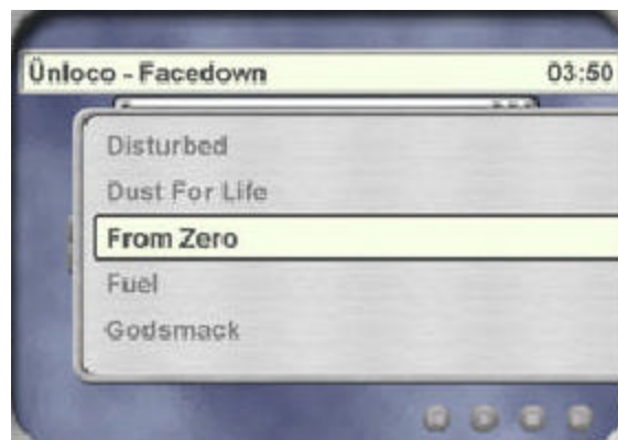
Figure 22. First revised interface for the carputer - Input from a remote control was now supported in addition to mouse control. The alphabetized list of songs shown in the center of the screen allows songs to be scrolled and selected with the remote.
