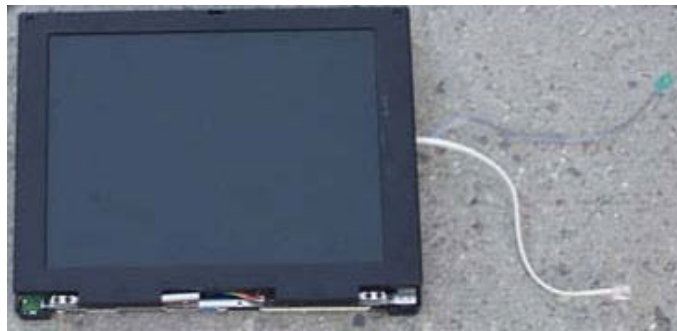
Figure 17. The carputer screen was reversed then placed back on the computer base.
