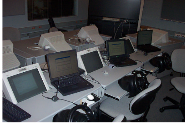
Figure 29. Image of the lab showing the three desktop computers used to run the simulator along side the three laptops used for the primary tasks.
