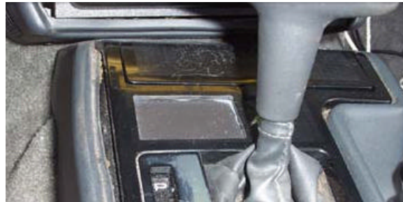
Figure 15. Image of the touchpad used in the carputer. Initially it functioned as a regular mouse, however, this was found to be unusable in a vehicle and was reimplemented as a graffiti character recognizer.
