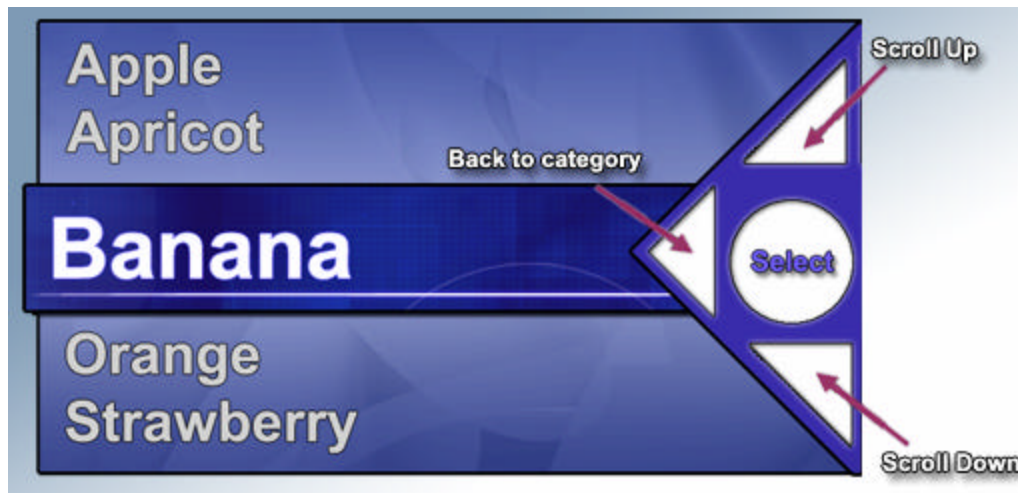
Figure 28. Touch screen interface for the carputer application. The scroll up and down arrows allow the list to be browsed, selections are made by tapping on the center select area. The list categories can be shown (if applicable) by pressing the back button.
