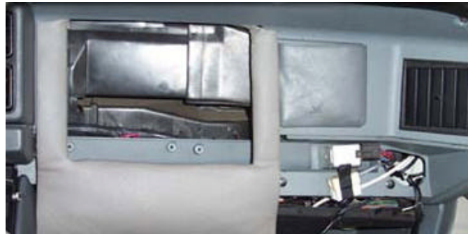
Figure 18. The carputer was installed on the passenger side of the car where the glove compartment once resided.
