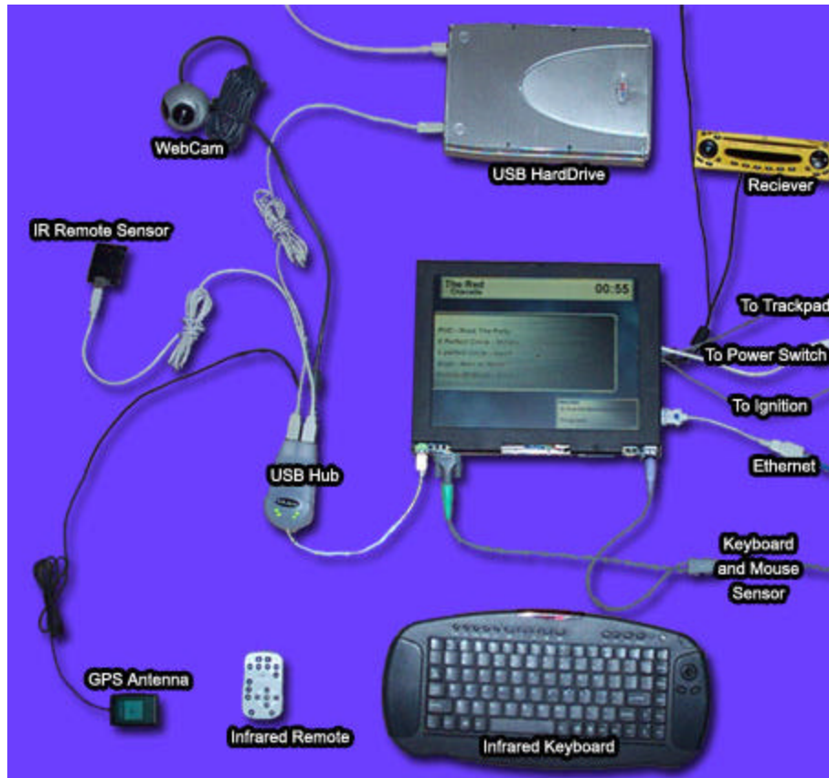
Figure 14. Carputer Hardware - All hardware shown is used to make the carputer function, the webcam is not yet implemented, but will allow for visual gesture control and speech recognition through its integrated microphone.
