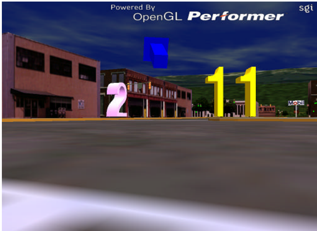
Figure 31. Screen shot from the driving simulator. The yellow numbers represent the speed of the driver, they turn green when the driver is going between 20 and 30 mph and red if 30 mph is exceeded. The pink 2 represents a checkpoint marker that the users must drive over to complete the course (Moldenhauer, 2003).
