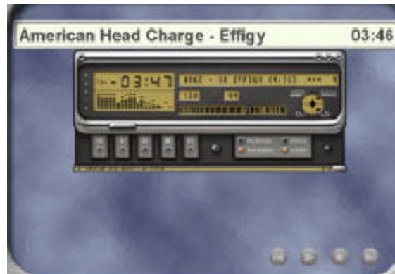
Figure 19. Initial interface for the carputer - winamp running in the center of the screen, the window at the very top shows the current playing song and time, the four buttons at the bottom control winamp. This interface offered litter in terms of usability in a vehicle.
