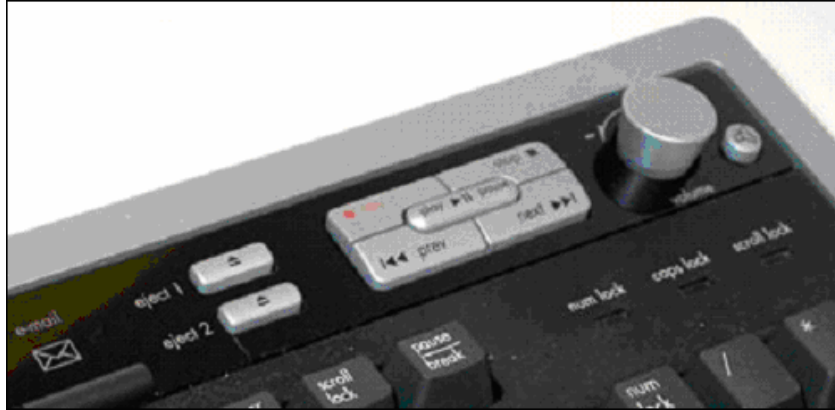
Figure 2. A Multimedia Enhanced Keyboard . The keys on the top of the keyboard can be used to control background tasks while working in another application (Shimpi and Anad Lal, 2003).
