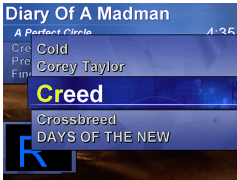
Figure 26. List selection in revision three of the carputer software. The graffiti recognizer in the bottom left of the screen shows the second recognized character as an "r". The list was shown when the first character "c" was received.
