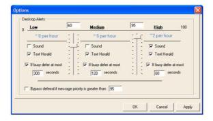
**Fig. 4.** Controls for a tool for specifying bounded-deferral policies for guiding alerting by the Priorities email triage system. Forecasts of the numbers of interruptions per hour for each class of email are displayed above each message-urgency column
